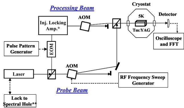
**Figure 1** Depiction of basic demonstrator system used. \* Injection locking optical amplifier; \*\*Frequency locking the laser linewidth to a transient regenerated spectral hole, technologies developed at MSU.
