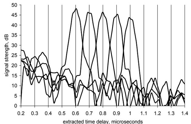
**Figure 2** Time delay over 0.6-1.0  $\mu$ s, showing 40 dB dynamic range. The processing sequences were repeated for 200 shots at 100 kHz, where each shot consisted a unique dynamic 512 bit pattern with 1 Gb/s BPSK modulation and its delayed replica.
