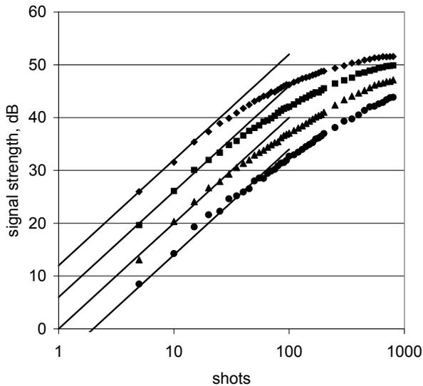
**Figure 3. Accumulation dynamics rms peak signal strength versus N programming shots for 2.5 mW programming power (top curve) and decreasing factors of 2 in power versus ideal coherent accumulation  $N^2$  (solid lines).**
