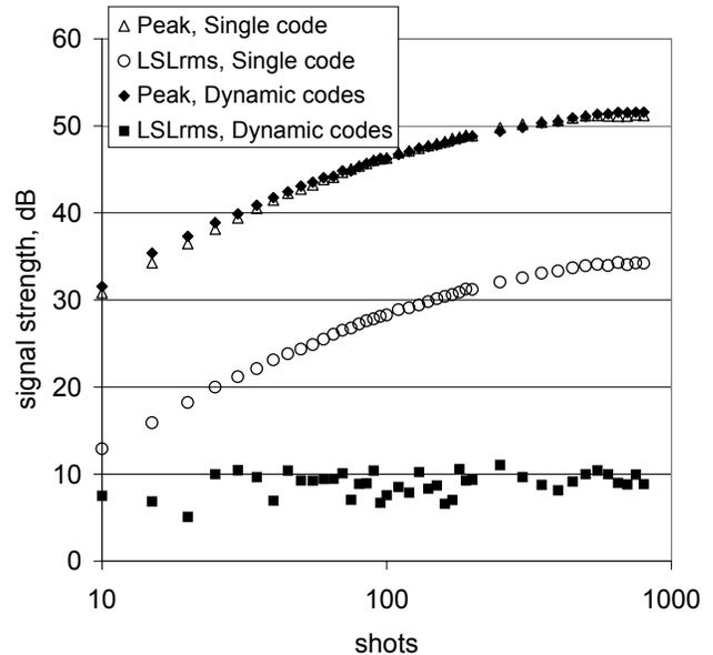
**Figure 4. The effect of agile processing with dynamic patterns is shown. The 'Peak' and the calculated rms left sidelobe 'LSLRms' values are plotted for both agile programming with dynamic patterns and accumulation with fixed pattern.**
