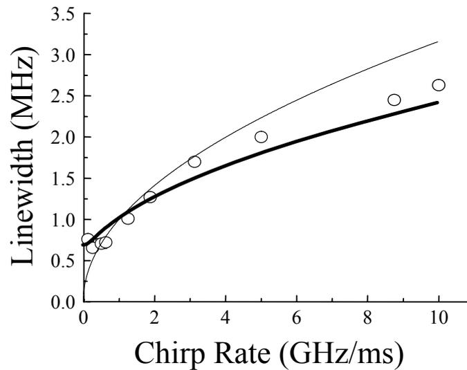
Figure 6. (a) Experimental (circles) and theoretical (thick line) evolutions of the linewidth (full width at half maximum) of a single-frequency readout signal versus chirp rate  $r$ . The thin line is  $r^{1/2}$ .
