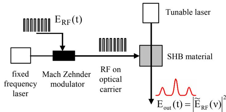
Figure 1. Basic principle of the spectrum photography analyzer.
